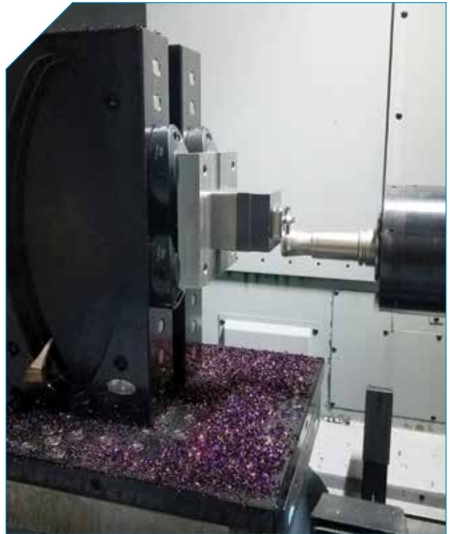
A four-axis milling machine processes a workpiece in Accu-Die's well-equipped shop.
